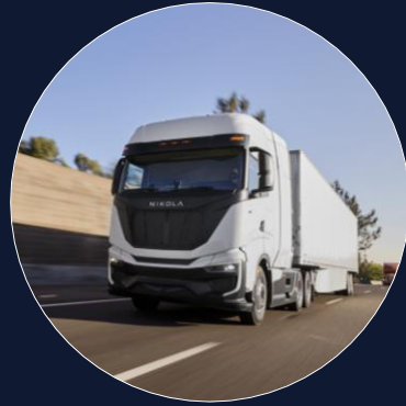
Nikola TRE FCEV heavy-duty truck now in production, first deliveries made in Q4'23 Range: up to 800 km Refuel time: 20 min or less
