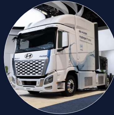
Hyundai XCIENT fuel cell truck ready for production – already launched in the United States Range: 720-800 km Refuel time: targets 30 min
